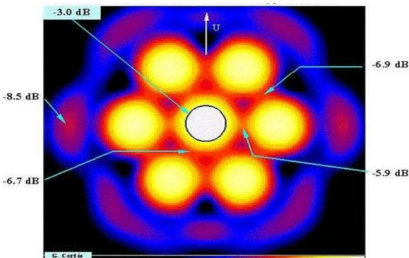
The ALFALFA survey exploits the Arecibo L-band Feed Array, dubbed ALFA. ALFA detects radio radiation at frequencies from 1225 to 1525 MHz. The array of feed horns allows for radio signal detection from 7 points on the sky simultaneously. ALFALFA uses overlapping drifts, so each pixel combines info from all 7 beams.
