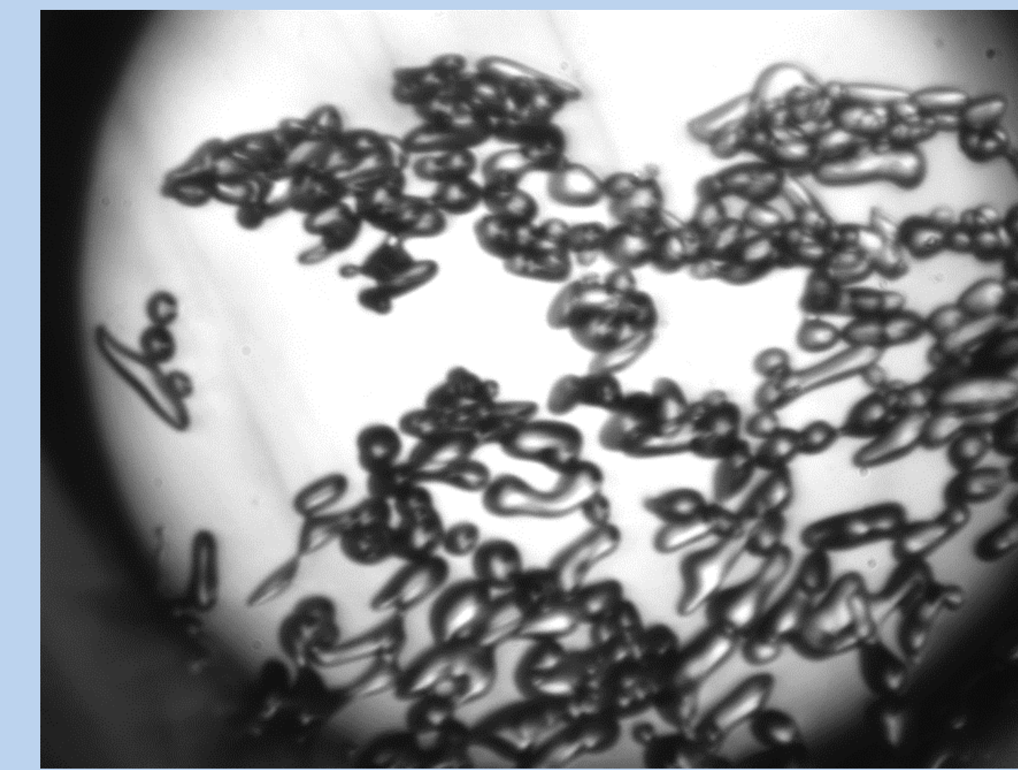
Fig. 6. Picture taken as the sample was melting, between points c and d. The crystals are falling downwards indicating that they are denser than water.
