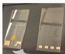
Inductive and Resistive sensor on glass slide
