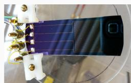
Sample Au thin film resistive sensor on a thermal oxide silicon substrate
