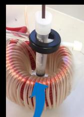
Use of fiber optic temperature sensor to measure Gd<sub>5</sub>Si<sub>4</sub> particles sample subjected to AMF
