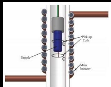
Schematic of pick-up coils
