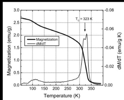
Magnetization (*M*) (thick line) and *dM/dT* (thin line) as a function of temperature (*T*) at a magnetic field of 0.01 T[1]
