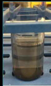
10 nm Gd<sub>5</sub>Si<sub>4</sub> Micro and Nano-particles in H<sub>2</sub>O, from Virginia Commonwealth University.
