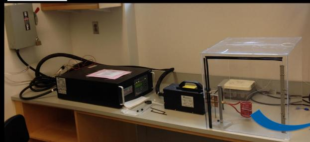
AMF generator (EasyHeat) setup with test magnetic field coil
